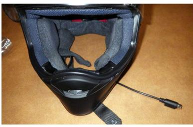
Helmet installation was easy. I secured the speakers in the speaker depressions with hot glue.
