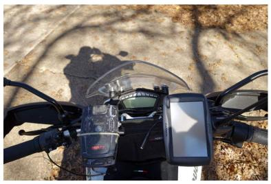
Just as easy to add to any bike. RAM 1" ball handlebar mounts hold the radar detector and GPS. The GMRS/FRS radio hangs on the bag.
