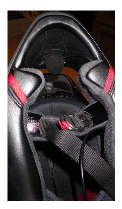
The microphone is attached with the two-side tape.
