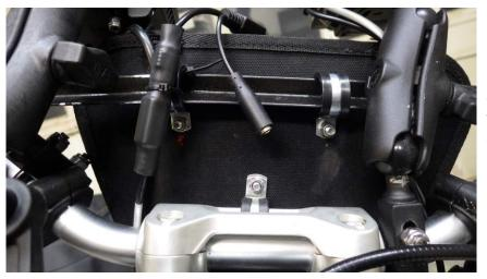
Cut small holes in the bottom of the bag to pass thru wires to my radar detector, GPS and B2B radio.
