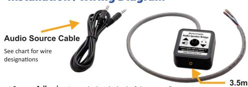
Converts audio from your bike speaker output for earphones or other use. Provides an isolation loop for both left and right channels. Balanced impedance correctly steps down voltage for a 3.5mm jack and built in load resistors protect your system.
